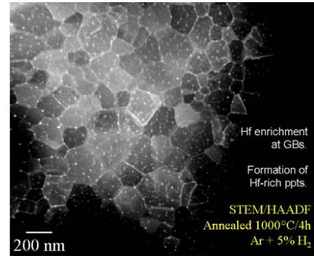
STEM-HAADF image of a high temperature NiAl-Hf intermetallic showing Hf segregation to grain boundaries and the formation of Hf rich precipitates.
